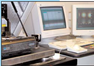
Scanning atomic force microscope (AFM) for surface metrology
