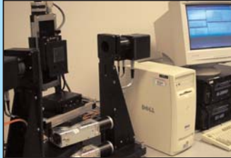
Spectroscopic ellipsometer for accurate thin film characterization
