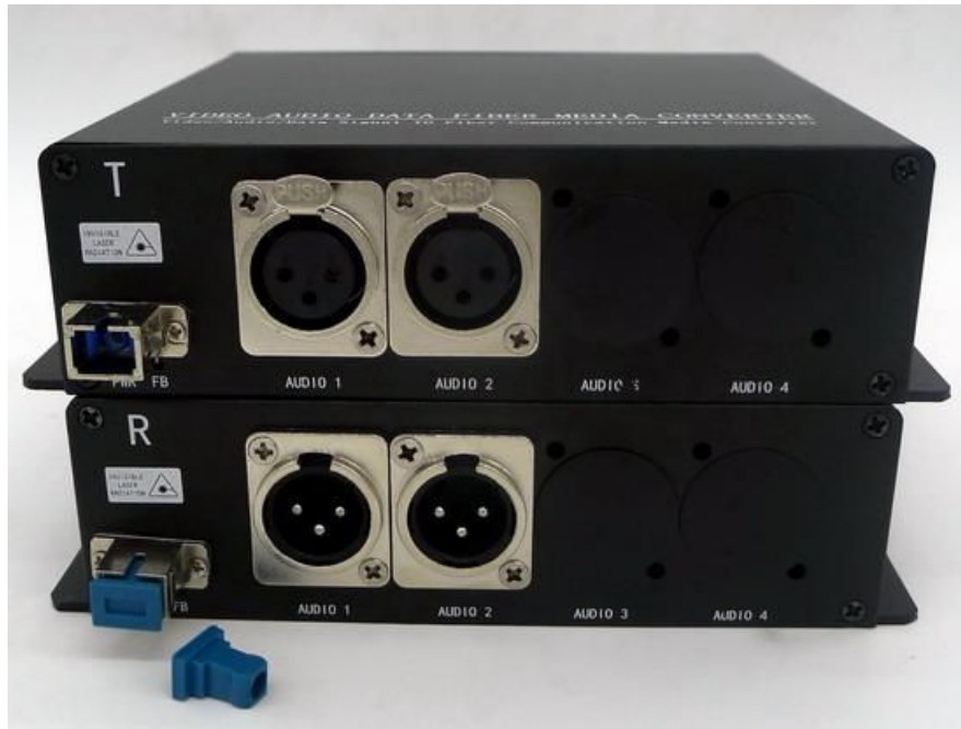
2 Channels Balanced Audio (XLR) To Fiber Optic
