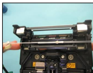
3. Transfer to heater and heat shrink splice sleeve.
