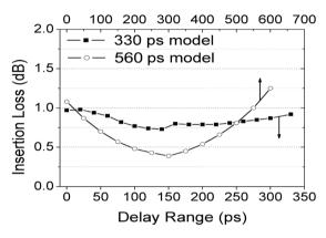
Figure 1. Insertion loss vs. optical delay.
