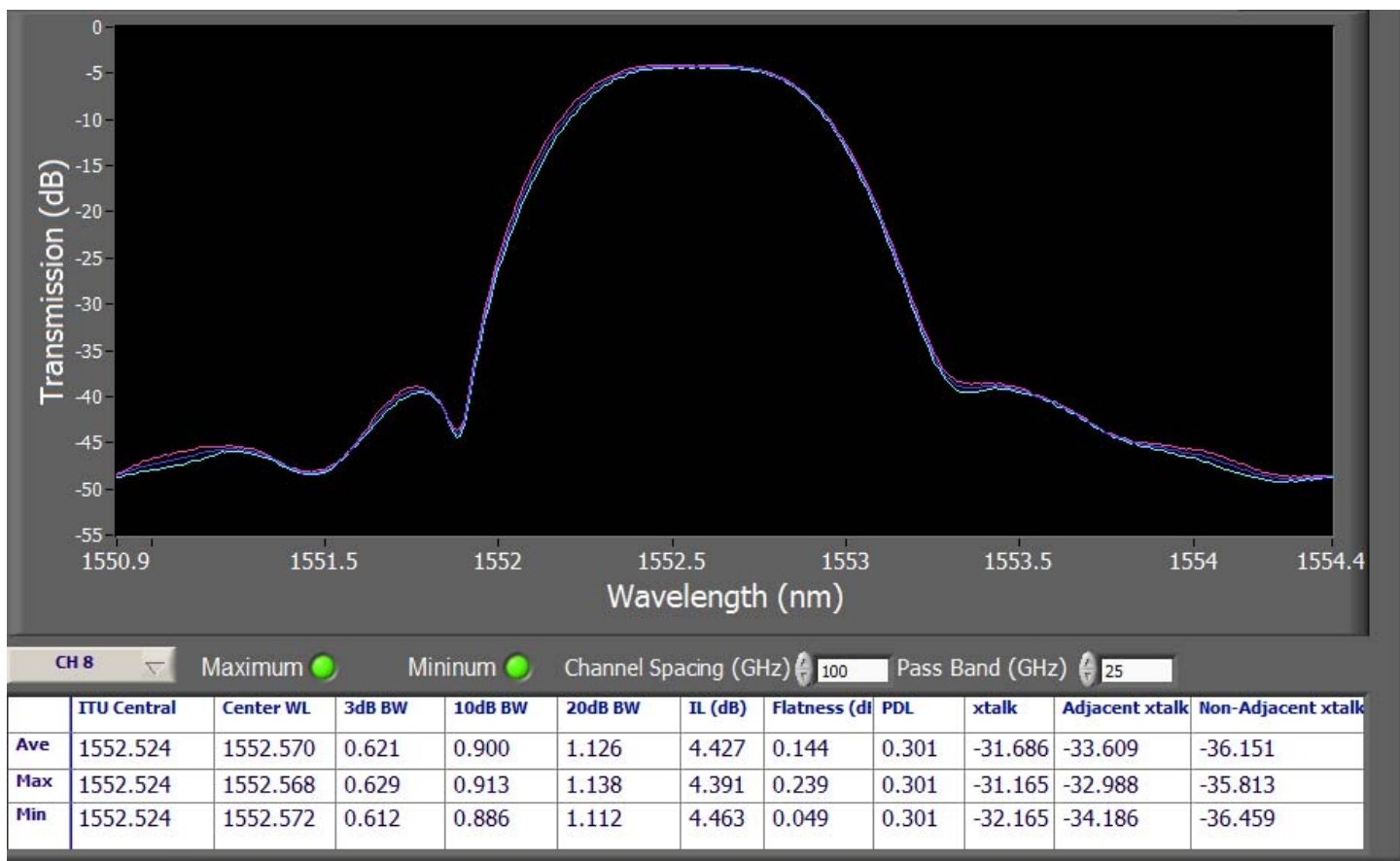
Figure 3 Detailed transmission vs. wavelength data for one channel of the same AWG. The plot shows the maximum, minimum, and average transmission vs. wavelength. The difference between maximum and minimum is an indication of the polarization dependent behavior for this device. The table shows the passband, flatness, and crosstalk information for this channel.
