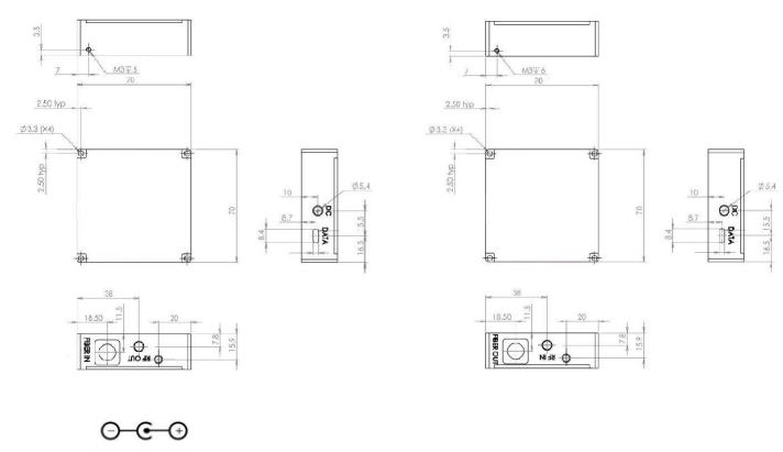
Connector: Positive center plug OD: 3.5mm, ID: 1.3mm, L: 9mm
