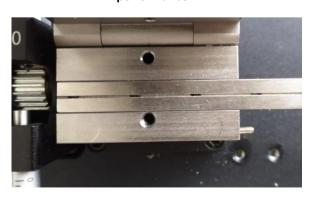
Different fiber holder adapters for different cladding diameter fibers (80~600µm)
