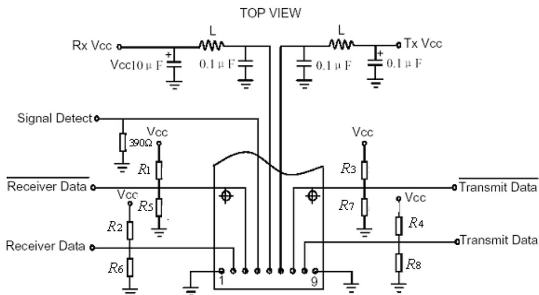
For :  $V_{cc}=5V$  ,  $R_1 = R_2 = R_3 = R_4 = 82\Omega$ ,  $R_5 = R_6 = R_7 = R_8 = 130\Omega$
