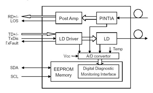
Figure 1: CCPXXD6-21-SDI Functional Block Diagram
