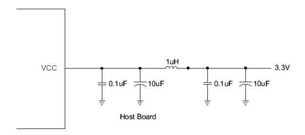
Figure 2: Recommended Host Board Supply Filtering
